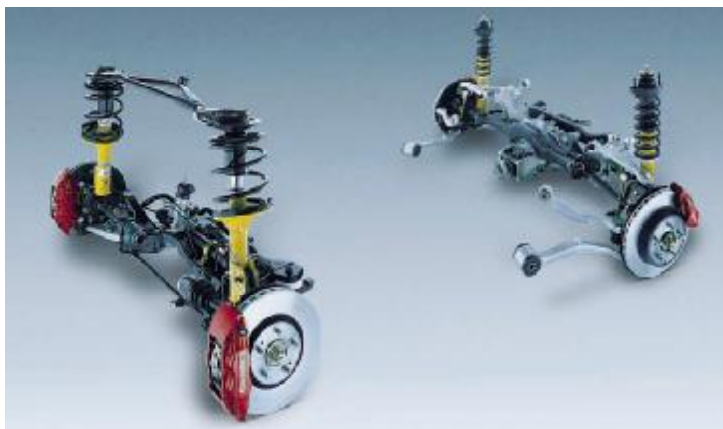
Front McPherson strut suspension, rear multi-link suspension, Brembo®* braking system/front 17" ventilated disc (4-pot) and rear 16" ventilated drum-in-disc (2-pot)
