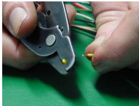
**Step 3:** Fit the heat shrink tube over the wire
