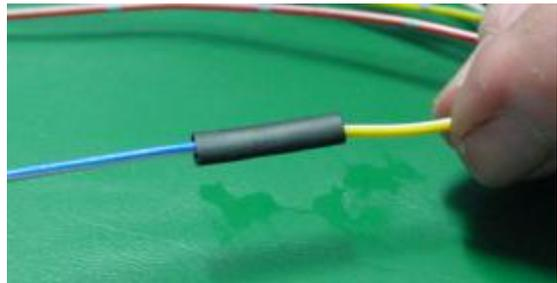
**Step 8:** Use heat gun to complete the heat shrink process. See example.
