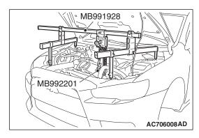
Install special tool MB991928 or MB991895 which is used during installation of transaxle assembly to hold the engine assembly. (Refer to GROUP 22A, Transaxle Assembly P.22A-127<M/T>), (Refer to GROUP 22C, Transaxle Assembly P.22C-341<TC-SST>)
