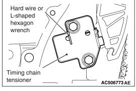
Remove the hard wire or L-shaped hexagon wrench fixing the plunger of the timing chain tensioner to apply tension to the timing chain.
