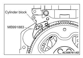
3. Use special tool MB991883 to secure the flywheel assembly in the same manner as removal.
