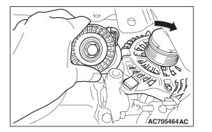
Loosen the mounting bolt of generator assembly lower part, and remove the mounting bolt of generator assembly upper part. Slide the generator assembly, and remove the auto-tensioner.
