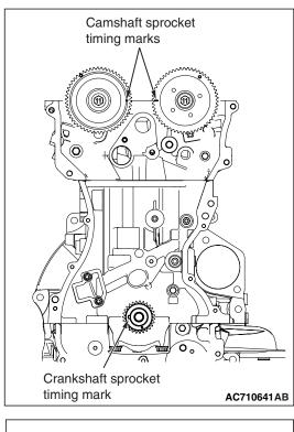
2. Align each sprocket timing chain mating mark with the link plate (blue) of timing chain to avoid slack of the timing chain tension side, and install the timing chain to the sprockets.
