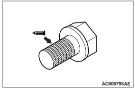
4. Apply a small amount of engine oil to the bearing surfaces of flywheel bolts and crankshaft tapped hole, and apply the sealant to the bolt threads of flywheel.
