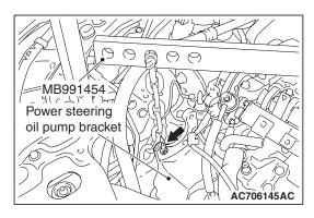
(3) Mount special tool MB991454 to the power steering oil pump bracket and the engine hanger, and set it to special tool MB991928 to support the engine and transaxle assembly.
