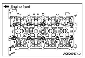
4. Loosen and remove the bolts in two or three steps in the order of number shown in the figure.
