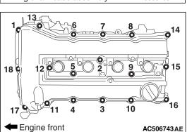
2. Apply sealant to the joint between the cylinder head and timing chain case assembly as shown in the figure and install the rocker cover assembly to the cylinder head.
