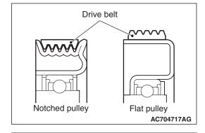
1. Install the drive belt to each pulley as shown in the figure.
