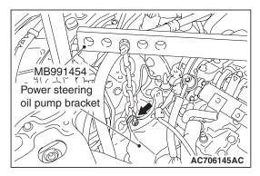
3. Set special tool MB991454 to the engine hanger and the power steering oil pump bracket.
