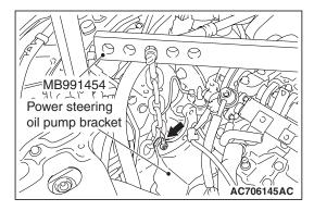
(2) Mount special tool MB991454 to the power steering oil pump bracket and the engine hanger, and set it to special tool MB991895 to support the engine and transaxle assembly.
