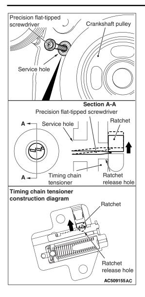
2. In the same manner as removal, insert the precision flat-tipped screwdriver through the service hole of the timing chain case, press up the ratchet of timing chain tensioner to unlock, and hold the unlocked timing chain tensioner.
