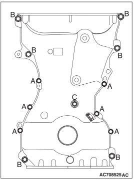
6. To the installation positions shown in the figure, tighten the timing chain case assembly mounting bolts to the specified torque shown below.
