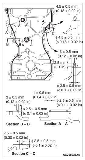
4. To the timing chain case assembly mating surface, apply the sealant with a width of  $2.5\pm0.5$  mm ( $0.1\pm0.02$  inch) and without a gap. However, with the "A" shown in the figure, apply the sealant with overlapping the diameter of  $4.5\pm0.5$  mm ( $0.18\pm0.02$  inch) or  $2.5\pm0.5$  mm ( $0.1\pm0.02$  inch) as shown in the figure.
