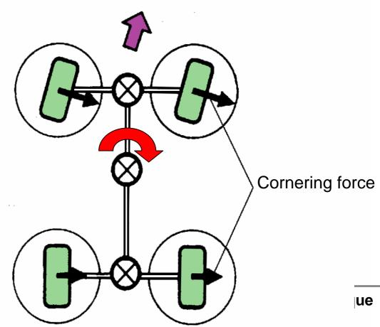
A Yaw Moment is the turning force placed on a vehicle when cornering. By controlling the Yaw moment, the cornering is improved
